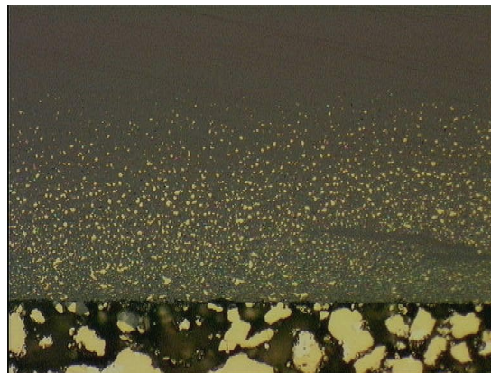
Fig. 2 Experimental simulation of DIS-i.s.s. using natural Fe-bearing and exsolution free sphalerite (grey) from St. Cristoph, Saxony. The crystal was embedded in synthetic Fe-rich i.s.s. (yellow, Fe/Cu=1.3) to run at T=573K over t=14d at a relatively high sulfur fugacity of the CuS/Cu 2-x S buffer. The experiment yields a fine-grained DIS-bearing rim (yellow) in the primary sphalerite crystal. Width of LM-micrograph: 125 \mu m, reflected light, Polar., oil.
