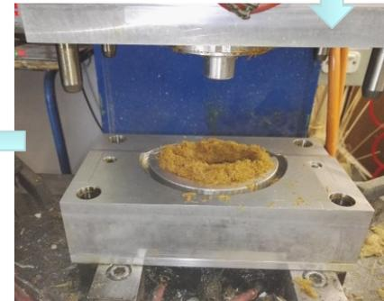
hot compression molding of natural fiber, bio-resin and bio-based flame retardant
